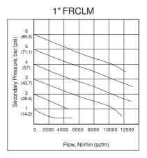
Flow graphs are for 40µm filterations only
